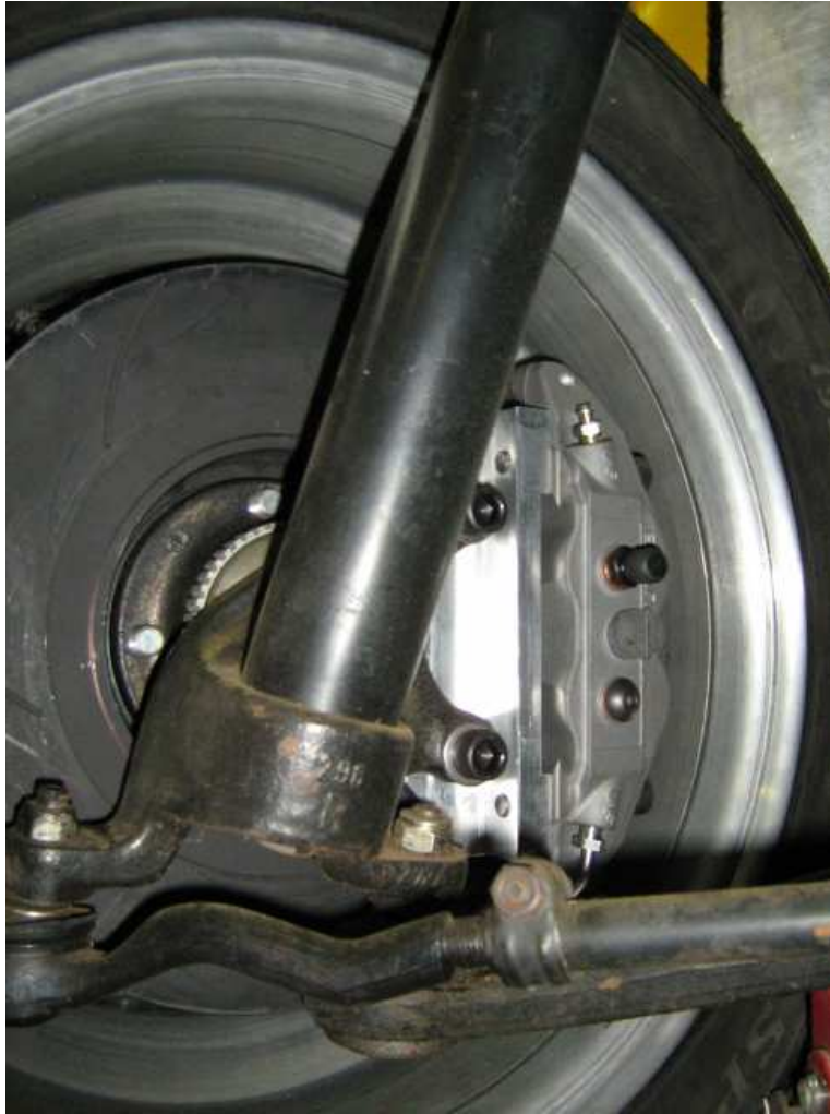
Figure 7: Showing the mounting bracket which attaches the Alcon caliper to the standard E30 caliper mounting points.
