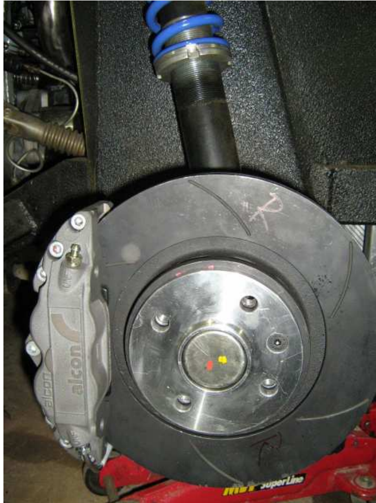
Figure 6: Showing the assembled Alcon caliper, Ferodo disc and Isotta wheel spacer attached to the E30 hub.
